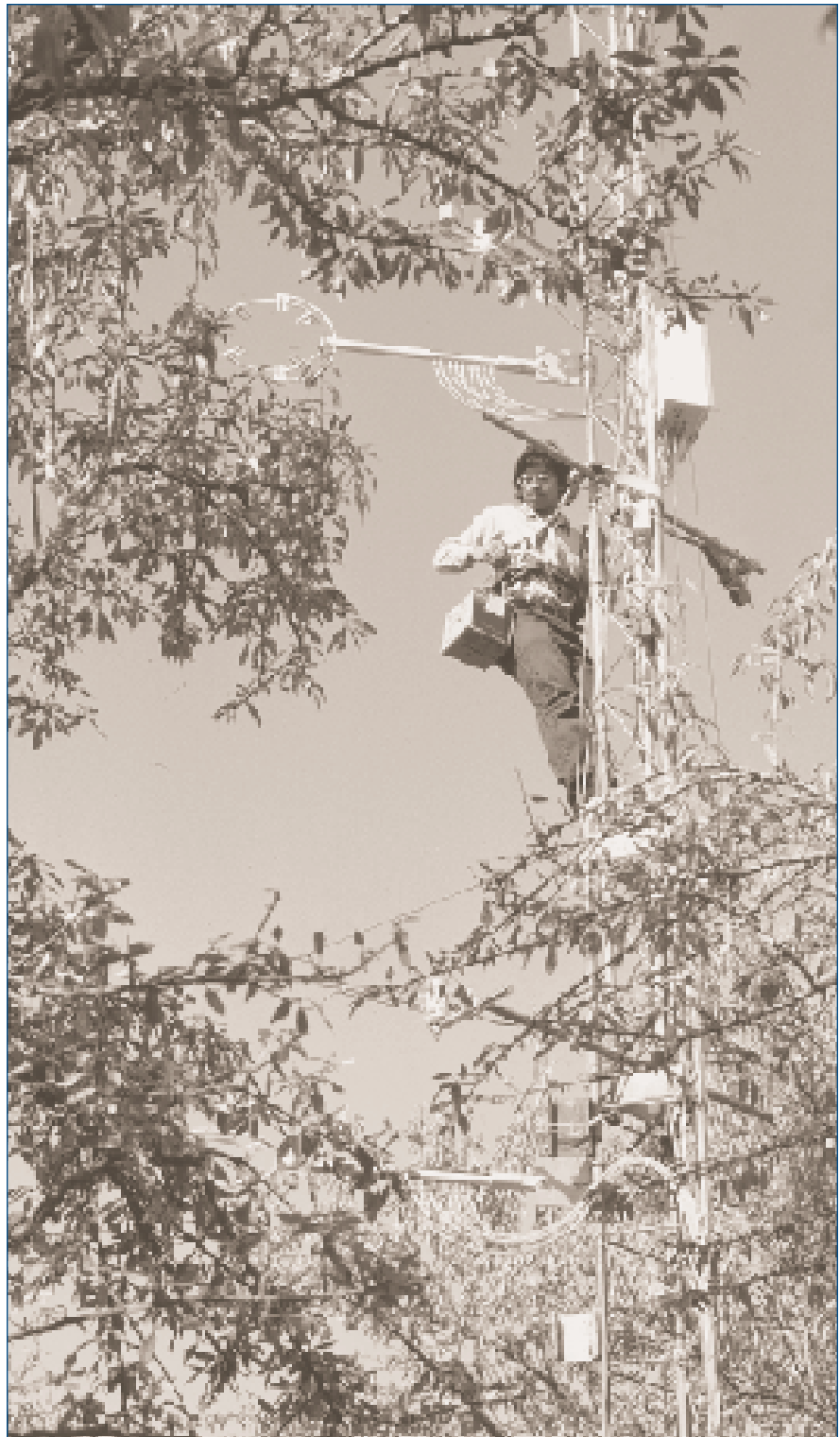
Professor Kyaw Tha Paw U installs a sonic anemometer on a tower to measure atmospheric turbulence in an almond orchard. Such measurements are used to determine vertical fluxes of water vapor and carbon dioxide.
